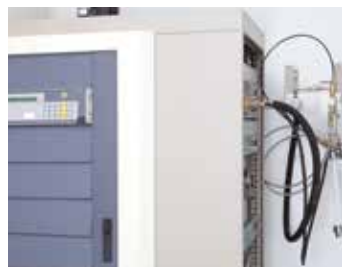
Pressure cycles Test on a system consisting of the pipe and fittings and subjected to 10,000 pressure cycles (from 1 to 30 bar) at 23 °C with a frequency of 0.5 Hz.
