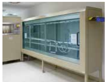
Thermal cycles Test on a system consisting of the pipe and fittings and subjected to 5000 temperature cycles (20 to 95 °C) of 30 minutes each with a pressure of 10 bar.
