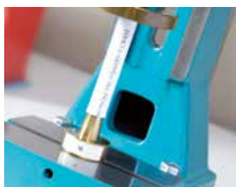
Enlargement Test Test performed both in production and in the laboratory to verify the quality of welds and the adhesion of individual layers.
