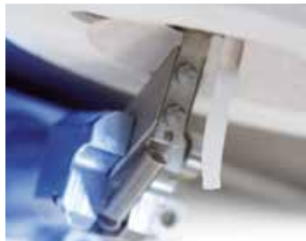
MFI (Melt Flow Index) Verify compliance of the polymer raw materials to be used.
