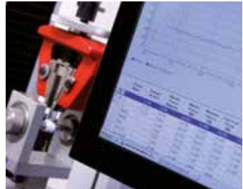
Peeling Test resistance to delamination between the inner layer and the aluminium.
