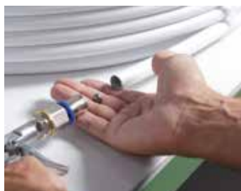
Ball Test To ensure that there are no occlusions or deformations on the inside of the pipe by using compressed air to pass a ball through the pipe.
