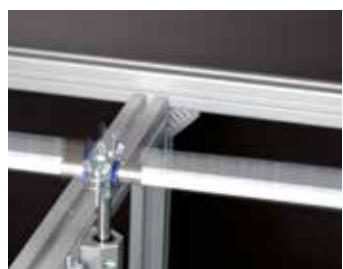
Vibration test Vibration test on a system consisting of pipe and fittings which is subjected to 330 alternating bending cycles with an internal pressure of 15 bar at room temperature.
